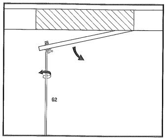
Hook the stowing pole bracket at the foot of the ladder and pull it outwards and downwards.
