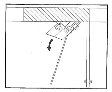
Care is needed when fully extending the ladder. Release the bottom locking catch 'A' and slide the front frame downwards until the top stops reach the upper guide brackets. Lower the ladder until the feet rest firmly on the floor. Engage locking catch 'B'. Ensure location plates are correctly located on the roller bar.
