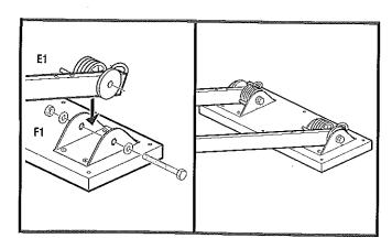
With the spring housing assembly in line with the ladder, fix it in position using six 40mm screws (F2).
