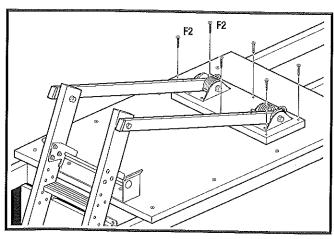
Release the top locking catch and slide the front section of ladder up until the latch engages. Pull or push the complete ladder assembly up into the loft until the anchor plates (D1) locate onto the roller bar. Fix the loop of each spring to the underside of the power arms using the J bolts (F3), washers and nuts (F4 & F5).
