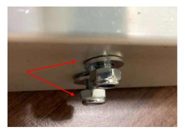
**Step 4** – Using 2 10mm spanners (not supplied), place a spanner on each end of the nut and bolt and tighten. Be mindful not to over tighten. Tighten all 4 nuts and bolts and check that the bearer bars are not loose and do not move. Please see photograph below;
