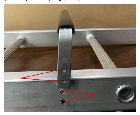
**Step 2** - Place 2 M6 x 40mm Bolts through the bearer bar and ladder stile. Repeat this process on each side of the ladder, 4 bolts in total per bearer bar. Please see photograph below;
